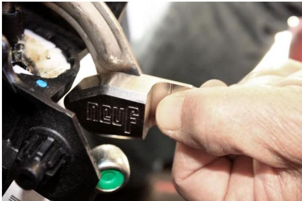
10. Install neu-f billet adapter onto lever, should be a snug fit. **NOTE:** Use Channel Lock pliers with taped jaws to squeeze on adapter. If adapter does not seat fully then more filing around edge may be required.
