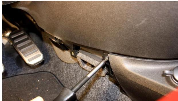
4. With cover removed, remove exposed T25 Torx screw.
