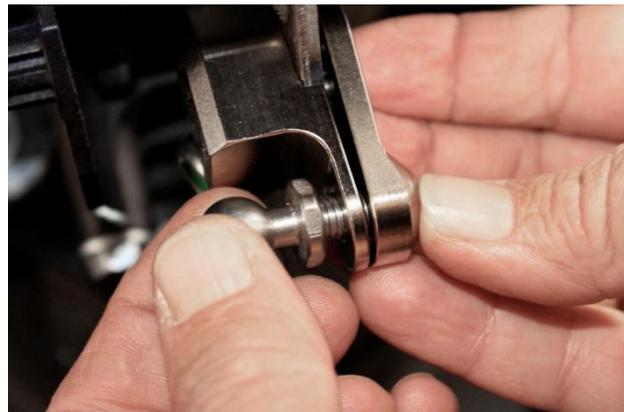
12. Install locking plate with cable ball end and M6x16 Socket Cap screw. Tighten evenly using 9/16" open end wrench and 5mm Hex Key wrench.
