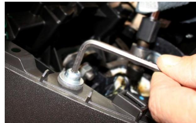
2. Remove the T25 Torx screw and 5mm Hex Key bolt from each side on the top edge of console.
