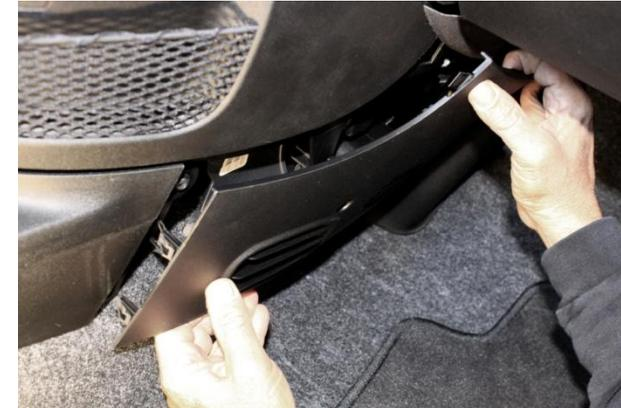
5. Remove the T25 Torx from passenger side lower cover then pull off.
