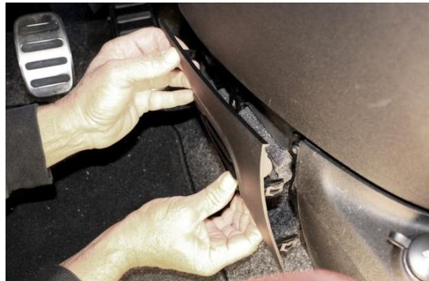
3. Remove the T25 Torx screw from driver side lower cover then pull off.
