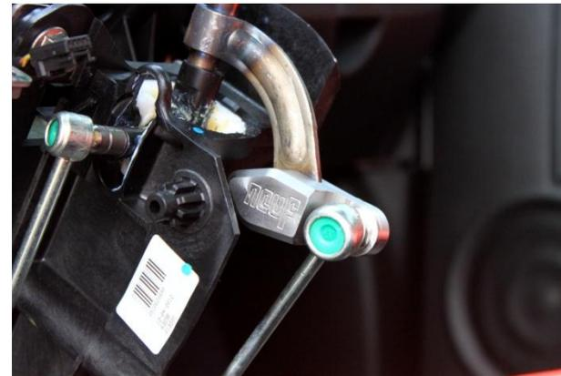
13. Grease ball and push on cable socket end. Check operation of shifting thru gears.
