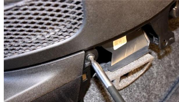
6. With cover removed, remove exposed T25 Torx screw.
