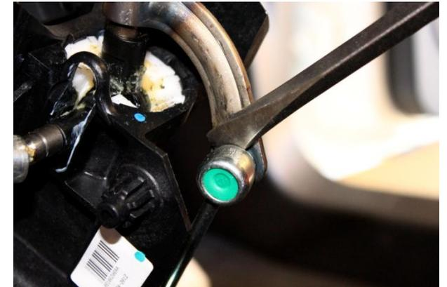
8. Using one or two screwdrivers pry off cable socket end from ball on shift lever.
