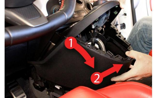
7. Tip back top of main console cover to separate from dashboard, and then lift out.
