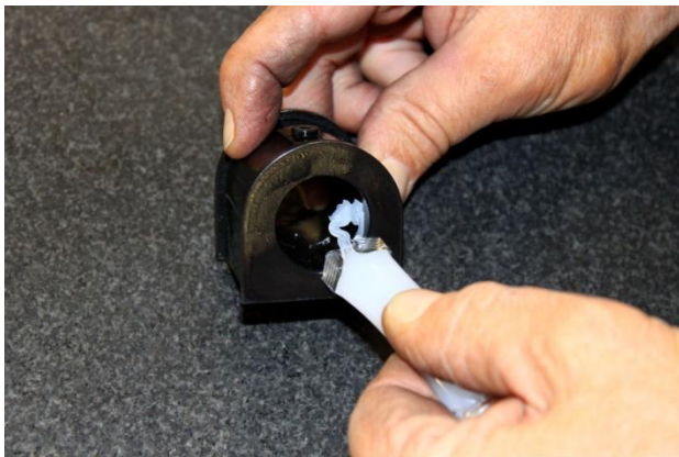
14. Grease urethane bushings with supplied grease and then install on inside of thrust washer on anti-roll bar.
