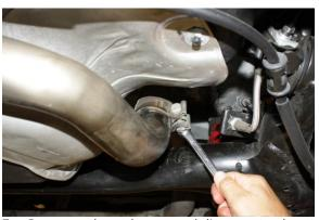
Remove exhaust hanger and disconnect exhaust at clamp connection just in front of rear axle beam.
