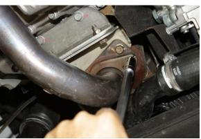
Remove the (2) front exhaust flange nuts using a 13mm socket.
