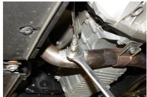
4. Using 22mm wrench, remove oxygen sensor.
