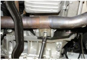
Remove exhaust support bolt at engine oil pan using 13mm socket.
