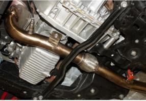
Install original metal gasket and put anti-seize compound on exhaust studs. Install NEUF front pipe with new flange nuts supplied and original bolt for exhaust support bracket into oil pan. Attach exhaust hanger. Put a little anti-seize on oxygen sensor threads and install into pipe.
