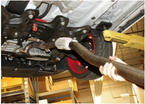
Flip over pipe and then remove from vehicle.
