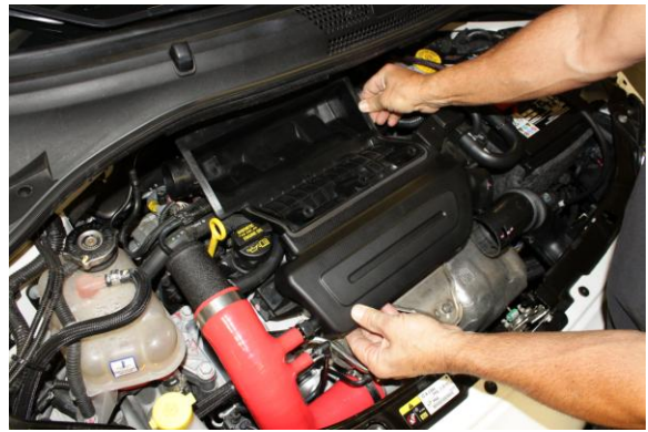
14. Install lower air filter box onto rubber mounts making sure vent hose is not being pinched off.
