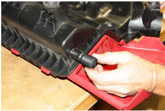
12. Cap port on air filter box using supplied vinyl cap.
