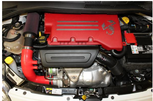
16. Install NEUF filter and original air filter box lid.
