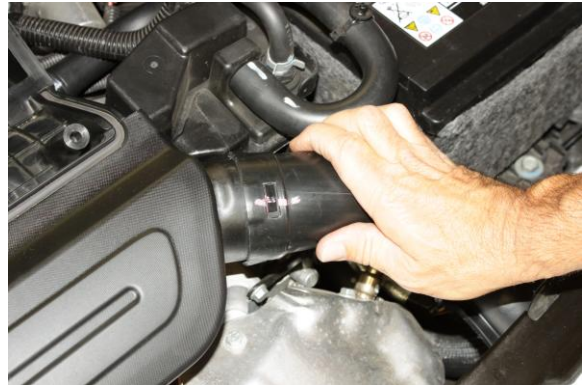
15. Connect front air intake duct.
