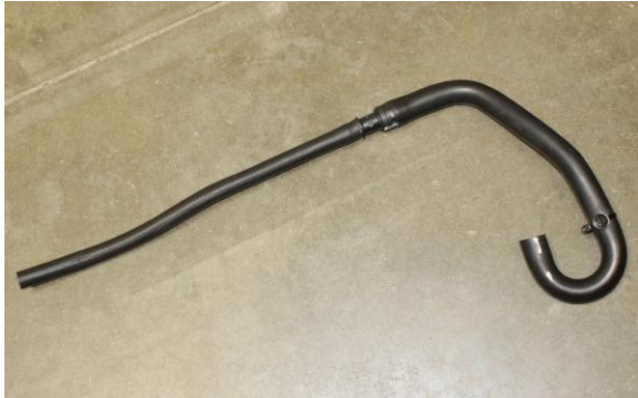
10. Attach supplied plastic union and 1/2" hose to original valve cover breather hose from air filter box.
