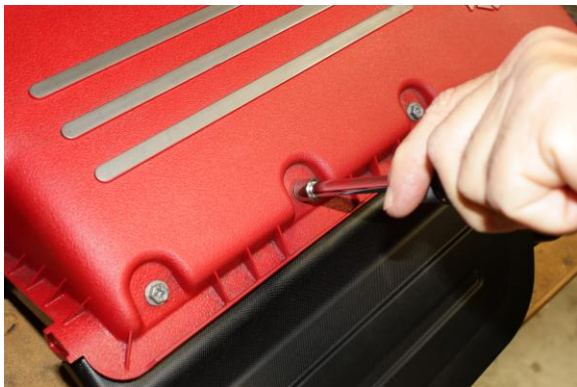
13. Unscrew air filter lid and remove filter.
