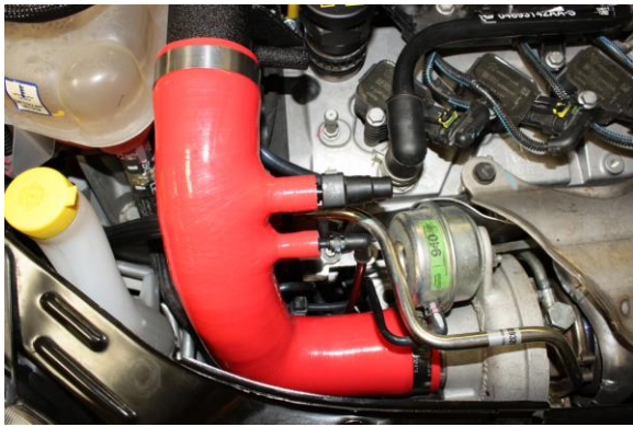
9. Attach vent lines and tighten hose clamps.
